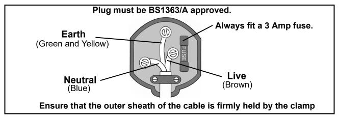
We strongly recommend that this machine is connected to the mains supply via a Residual Current Device (RCD). If in any doubt, consult a qualified electrician. DO NOT attempt any repairs yourself.
